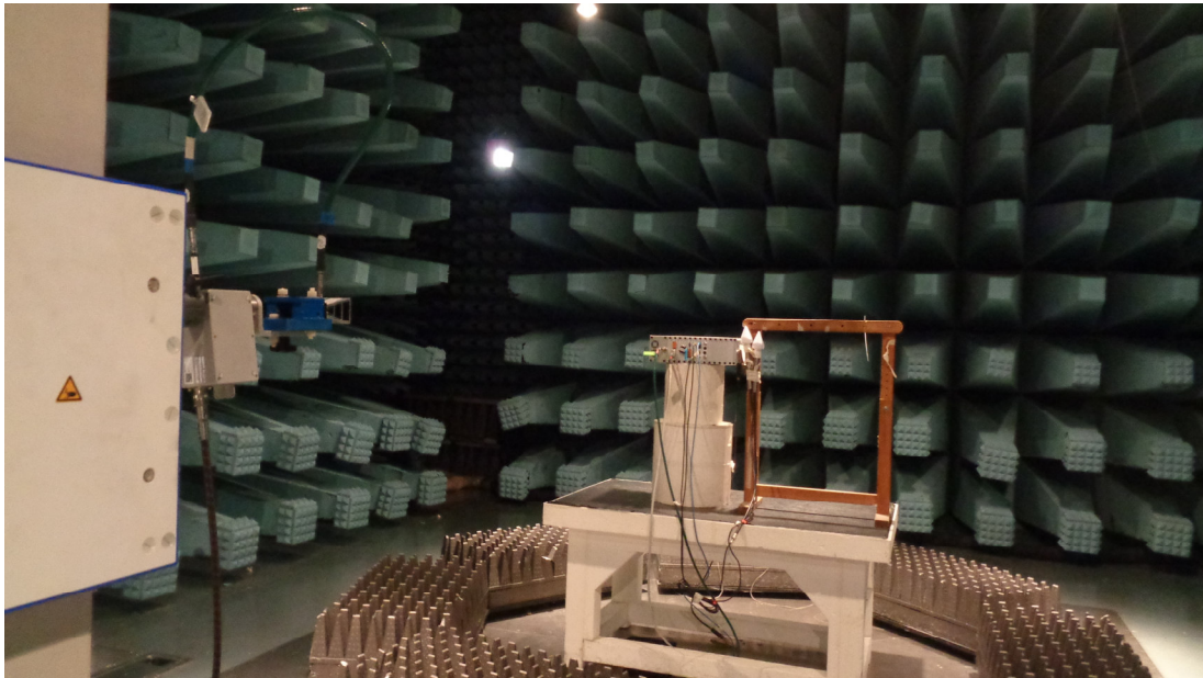
Set-up photo for radiated tests above 1 GHz photo
