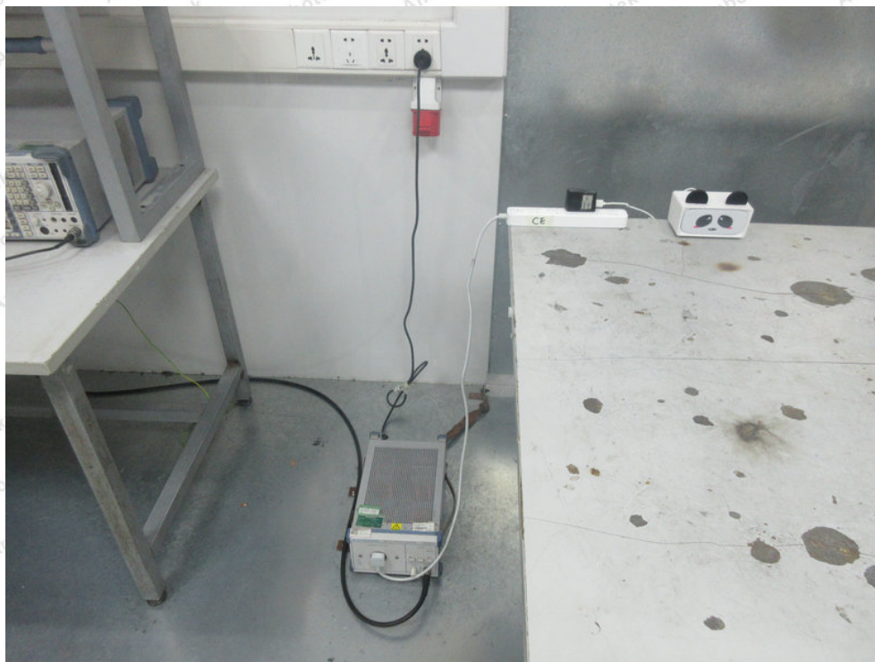
Photo of Conducted Emission Measurement
