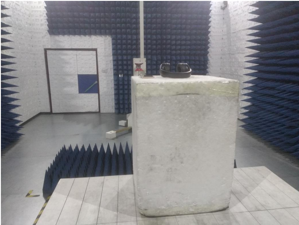
RADIATED EMISSION TEST SETUP ABOVE 1GHZ
