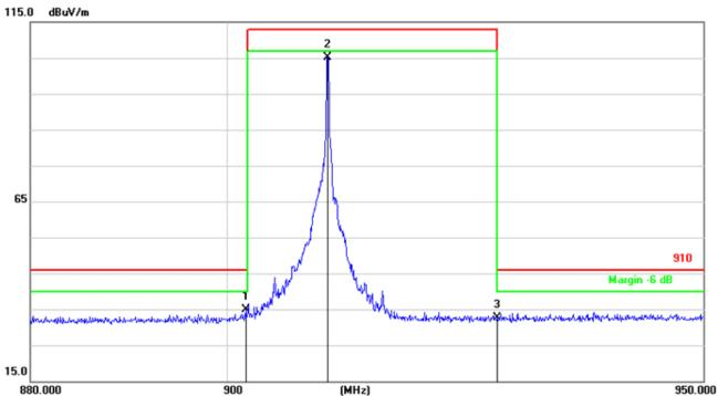
No. Reading Result Limit Remark Frequency Correct Margin (dBuV/m) (MHz) (dBuV/m) Factor(dB/m) (dBuV/m) (dB) 1 901.8400 36.43 -1.49 34.94 46.00 -11.06 peak 2 -7.84 910.3100 106.58 -1.42 105.16 113.0 peak 3 34.02 -1.28 32.74 46.00 -13.26 928.0000 peak
