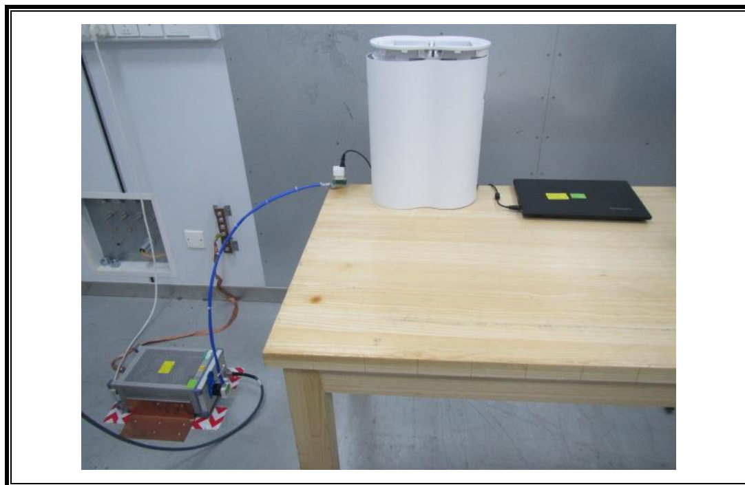
POWERLINE CONDUCTED EMISSIONS MEASUREMENT SETUP
