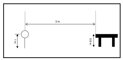
Radiated emission setup, below 1 000 MHz
