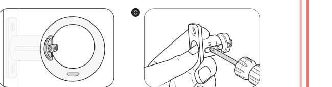
D. Fasten the bolt with the provided bolt plate screws. Do not use power tools at any point during the installation. Power tools will strip the screws.
