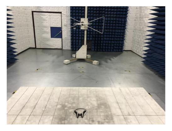
RADIATED EMISSION TEST SETUP ABOVE 1GHZ
