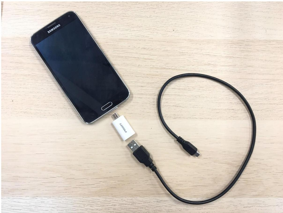
3. **Important!** Please make sure the Node is switch off before connecting to your Android phone. 4. Plugin micro USB end to the Node.
