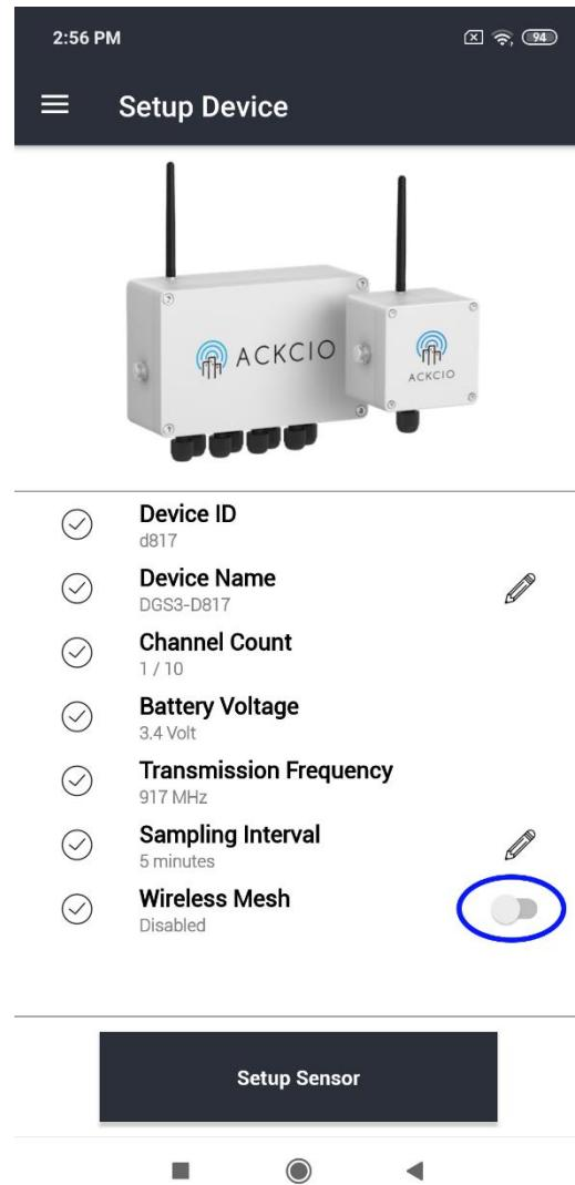
(iii) <Optional Step> If Wireless Mesh (Relay) function is to be deployed, click on "Wireless Mesh" toggle button to enable. Once done, click on “Setup Sensor”, you can now configure the sensor settings.
