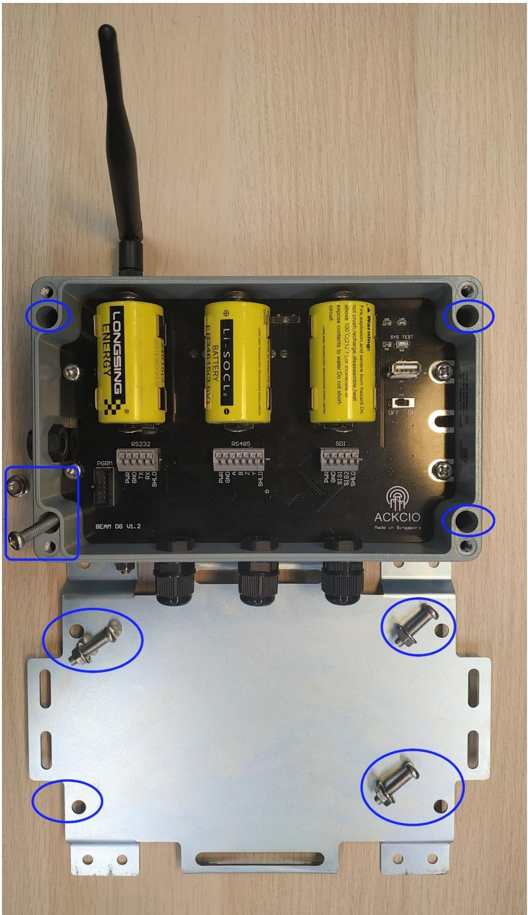
Use four screws and nuts to attach the node to the bracket
