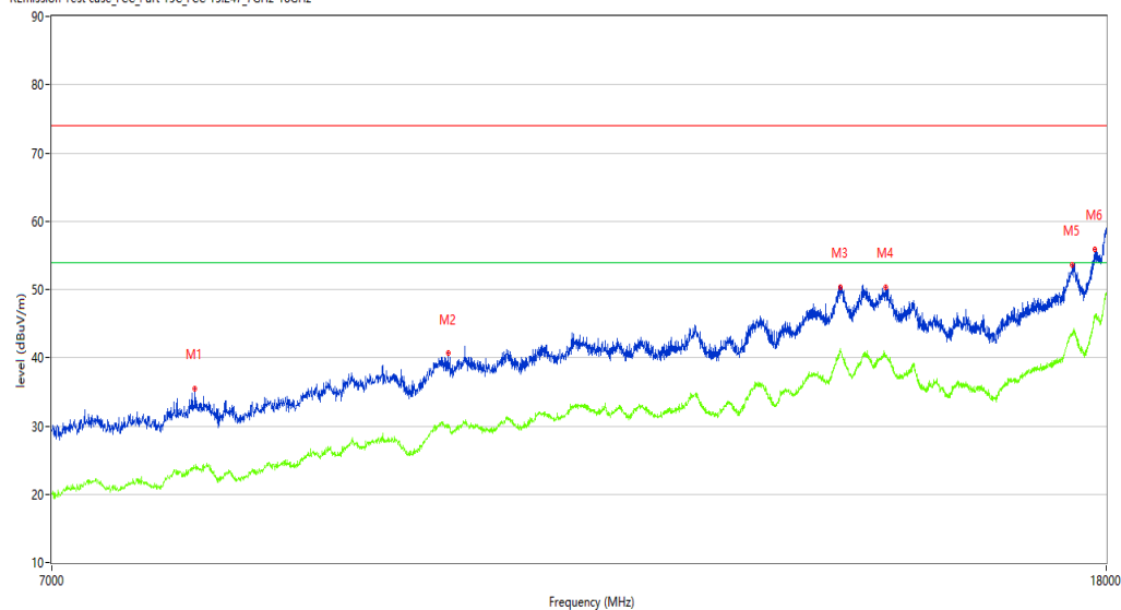
REmission Test case_FCC_Part 15C_FCC 15.247_7GHz-18GHz
