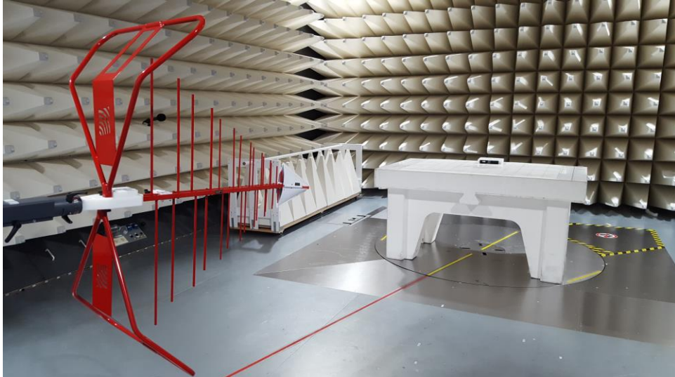
Figure B3. Low Range Radiated Emission Set up
