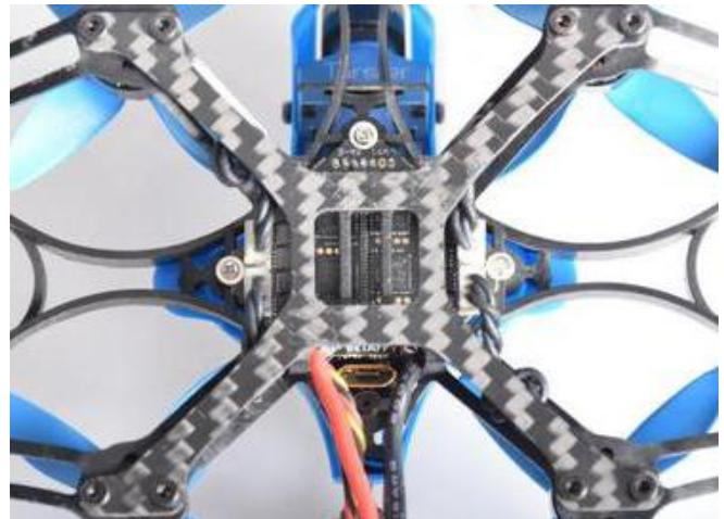
The stiffener brace of carbon fiber can reinforce the Beta85X frame, avoid instability caused by too strong power when Beta85x is flying.
