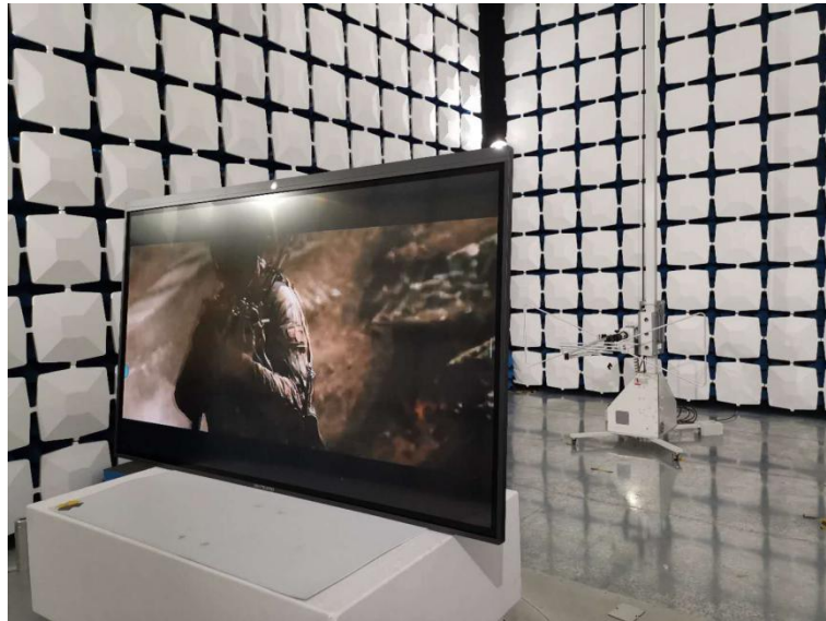
Blow 1GHz for radiated emission test setup
