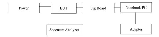
6.5.2 Radiated Emission and Conducted Emissions measurement Setup
