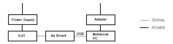
6.5.3 Radiated Emission measurement Setup for below 30 MHz
