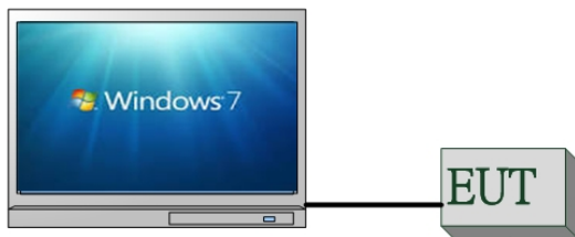
Fig. 2-1 Conducted (Antenna Port) Emission Configuration
