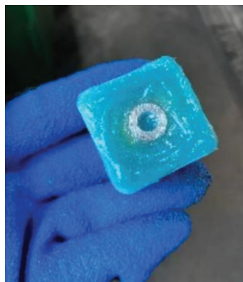
Figure: DynaLogger installation with glue fixation
