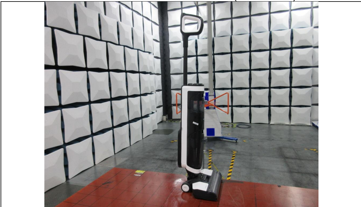
RADIATED RF MEASUREMENT SETUP (30MHz~1GHz)
