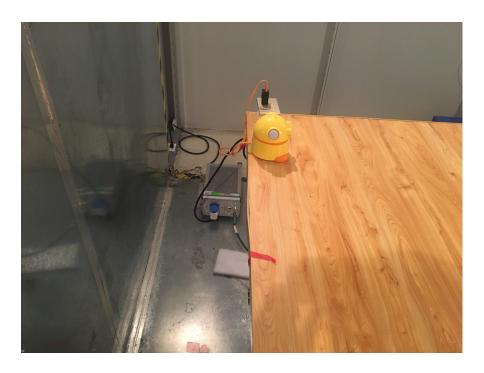
**Radiated Emissions (9kHz-30MHz)**
