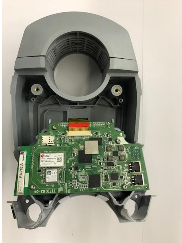
Figure 12: EUT Picture – Rear View – PCB ribbon cable connection
