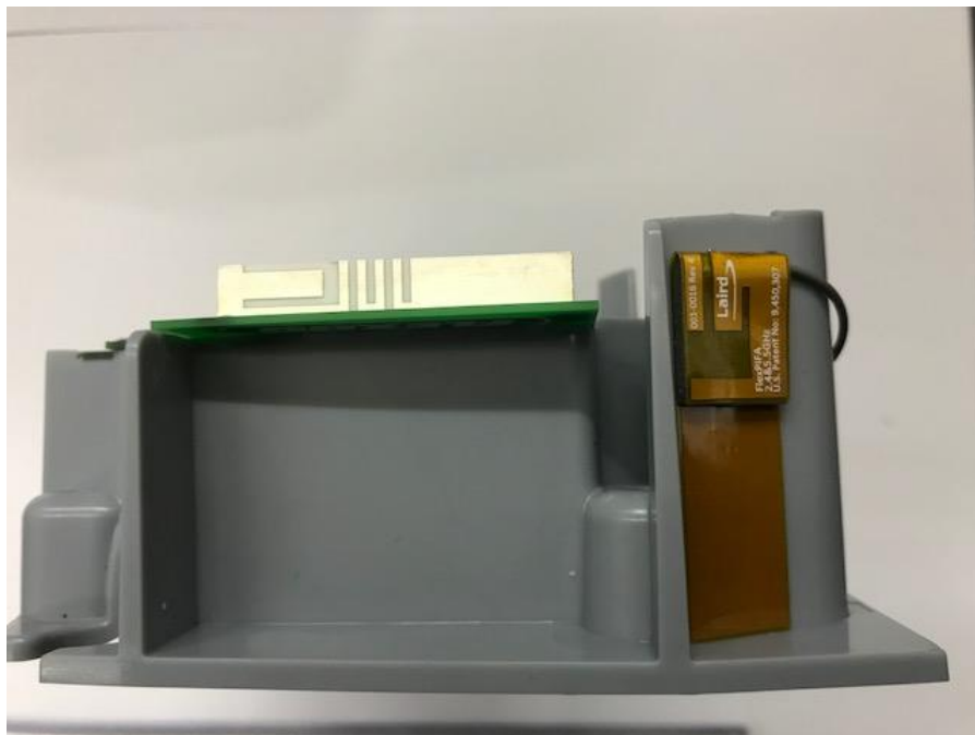
Figure 17: EUT Picture – WiFi\BT antenna 2 (right side) – Cellular antenna (upper side)
