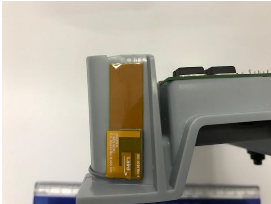
Figure 16: EUT Picture – WiFi\BT antenna 1 - Detail
