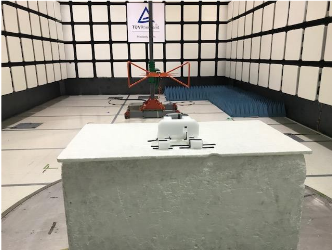
Figure 20: 30 - 1000 MHz Radiated Emission Test Setup – Rear View
