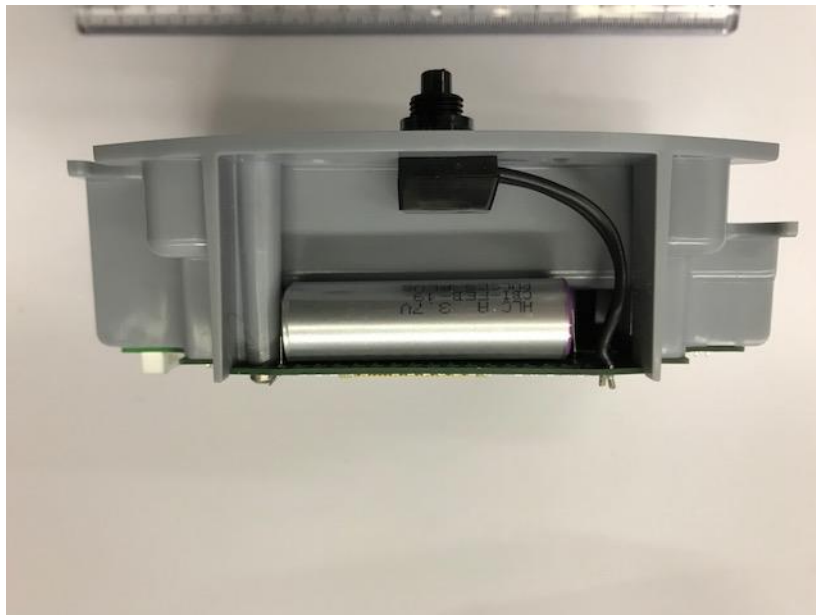
Figure 11: EUT Picture – side view – power capacitor and On\Off button
