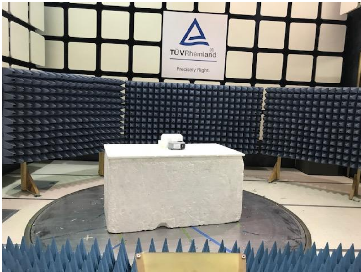
Figure 22: 1 – 18 GHz Radiated Emission Test Setup – Front View – EUT Horizontal
