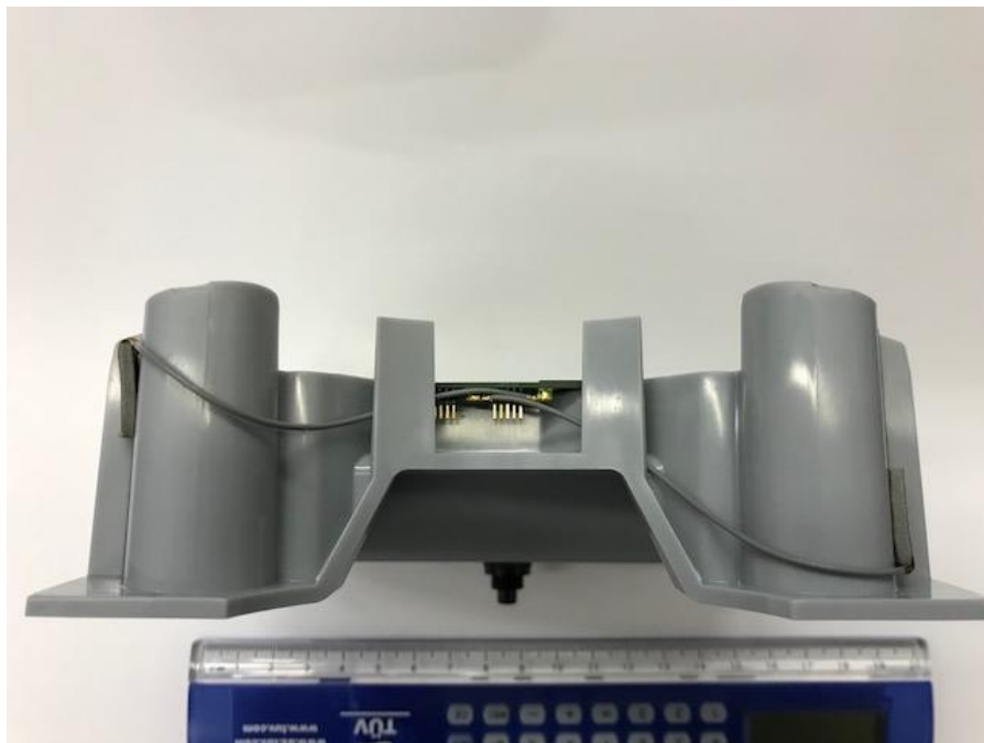
Figure 15: EUT Picture – U.FL connection and WiFi\BT antenna cabling (Note: BT\WiFi antenna visible left and right side)
