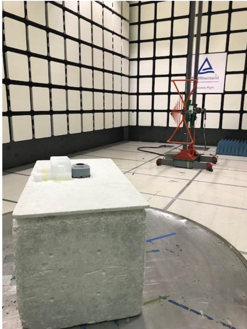
Figure 19: 30 - 1000 MHz Radiated Emission Test Setup – Front View – EUT Horizontal
