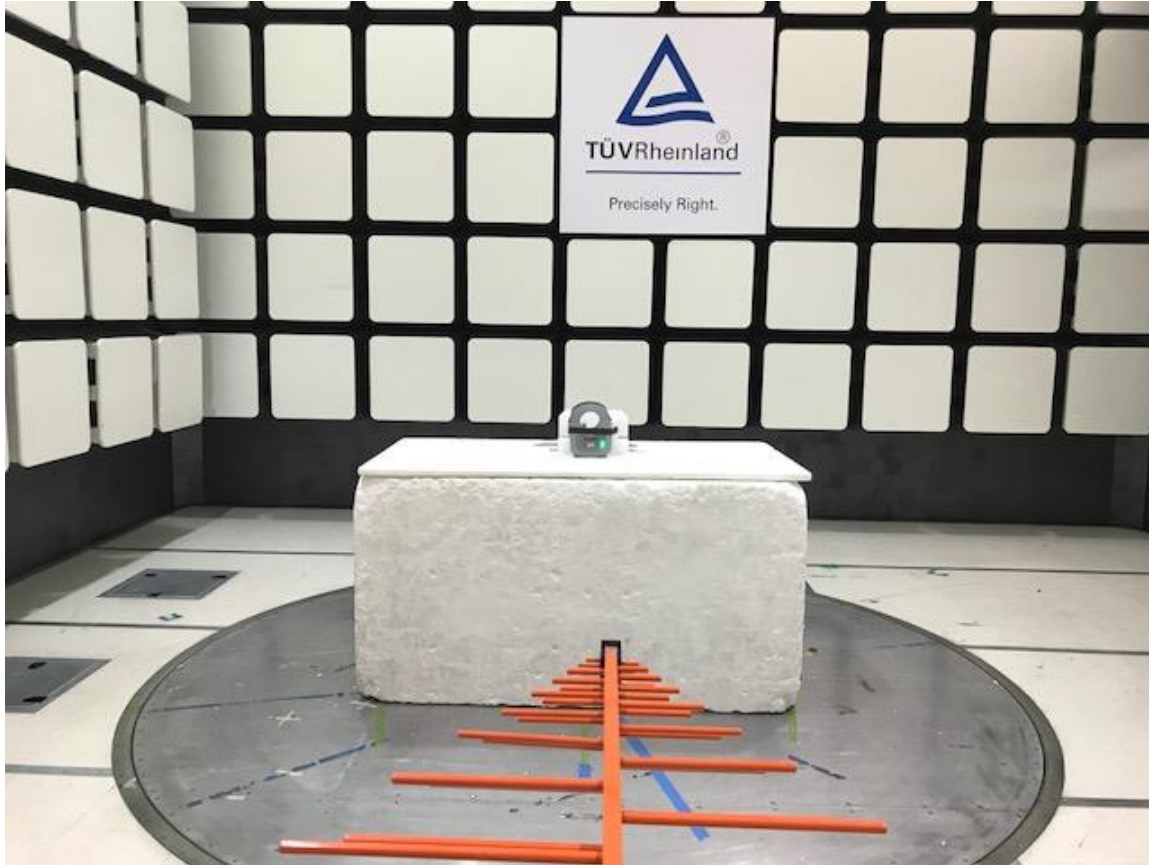
Figure 18: 30 - 1000 MHz Radiated Emission Test Setup – Front View – EUT Vertical
