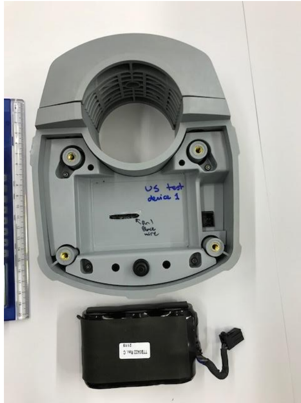
Figure 10: EUT Picture – Rear View – temporary serial programmer access (Not present in final design)
