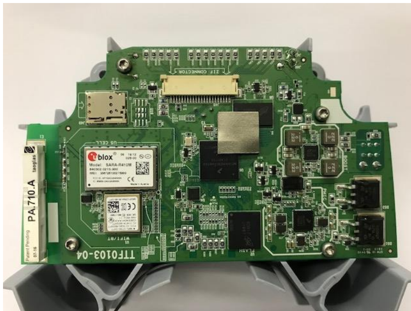
Figure 13: EUT Picture – PCB Front (Note: Cellular antenna PA.710.A – left side)
