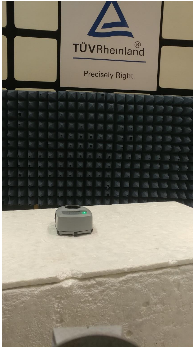
Figure 24: 18 - 30 GHz Radiated Emission Test Setup – Front View
