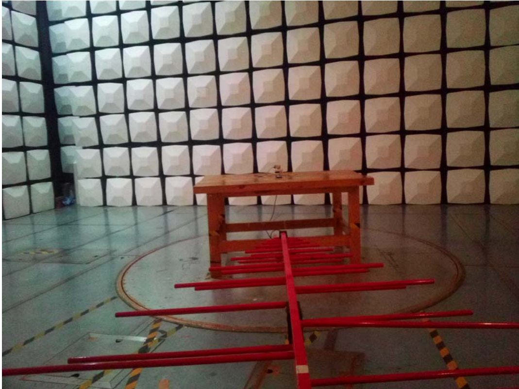
Radiated Emission Above 1GHz View
