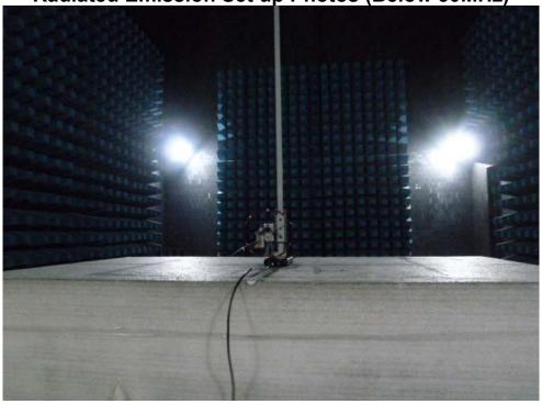
Radiated Emission Set up Photos (Below 1GHz)
