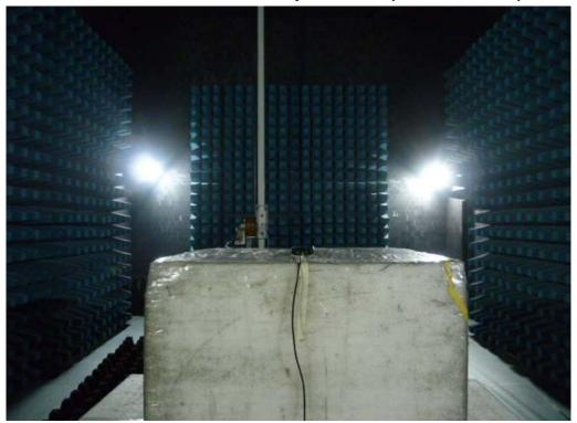
Radiated Emission Set up Photos (Front View)
