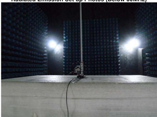
Radiated Emission Set up Photos (Below 1GHz)
