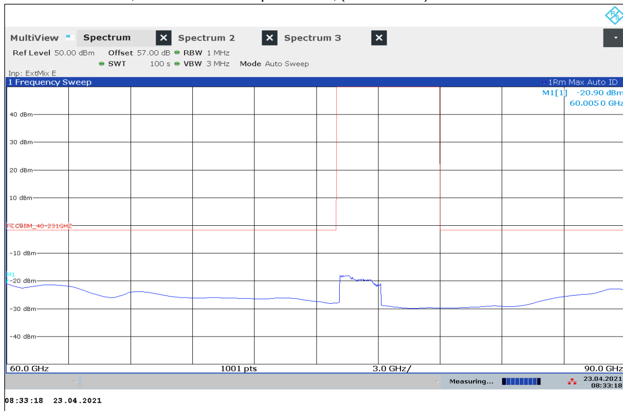
Plot 17: 60 GHz – 90 GHz, vertical / horizontal polarization, (mode5_5169)
