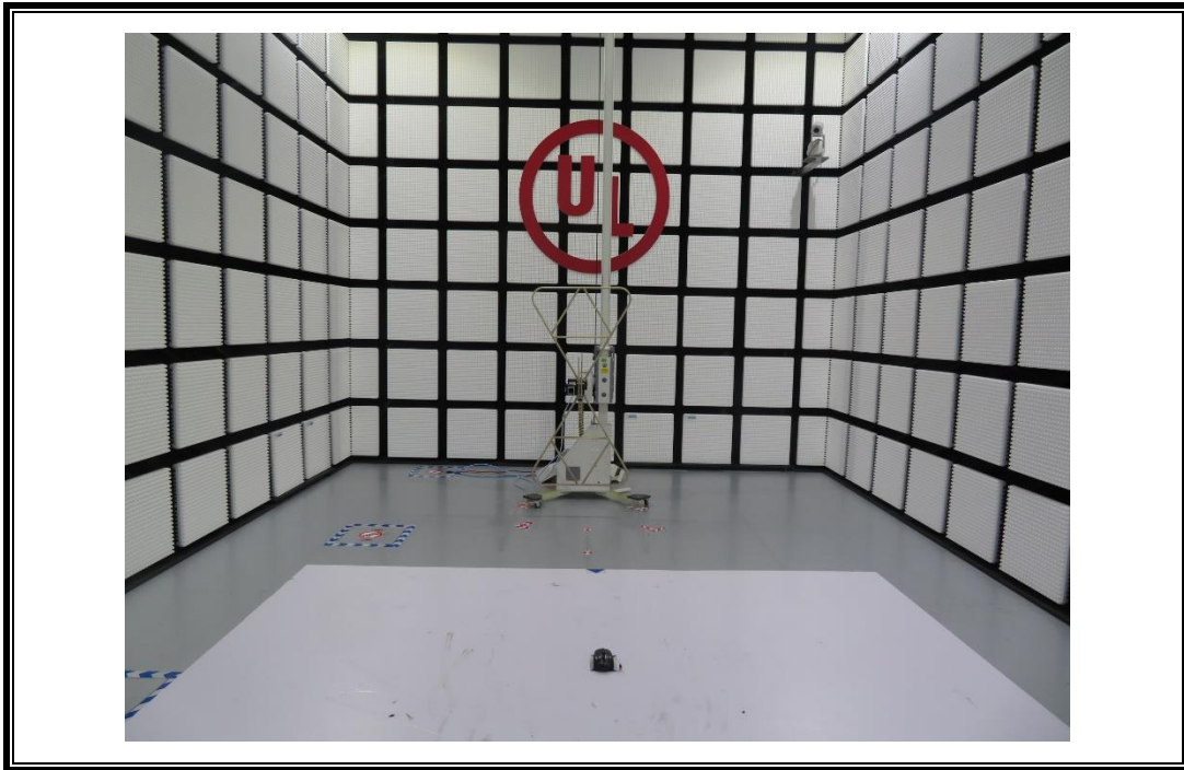
RADIATED RF MEASUREMENT SETUP (30MHz ~ 1 GHz)
