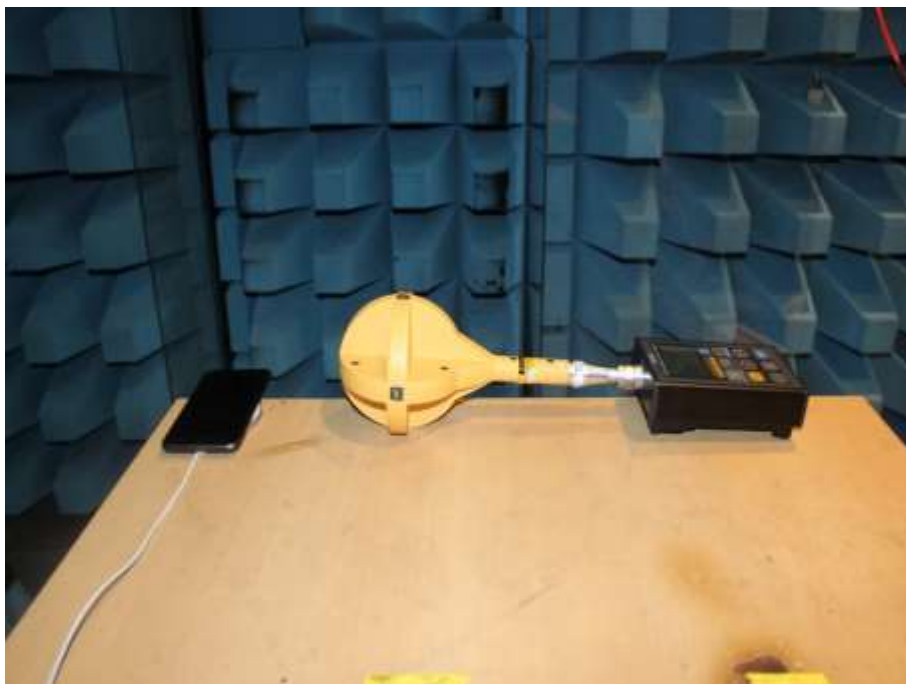
Photograph 4: Set-up for RF Exposure
