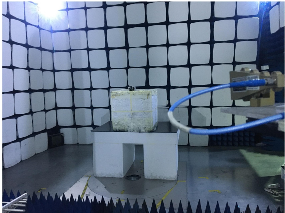
Radiation Emission Test Setup (Above 18GHz)
