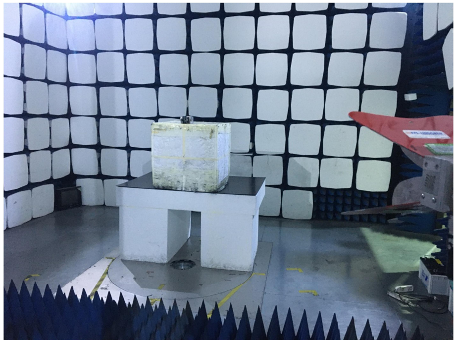
Radiation Emission Test Setup (1GHz to 18GHz)
