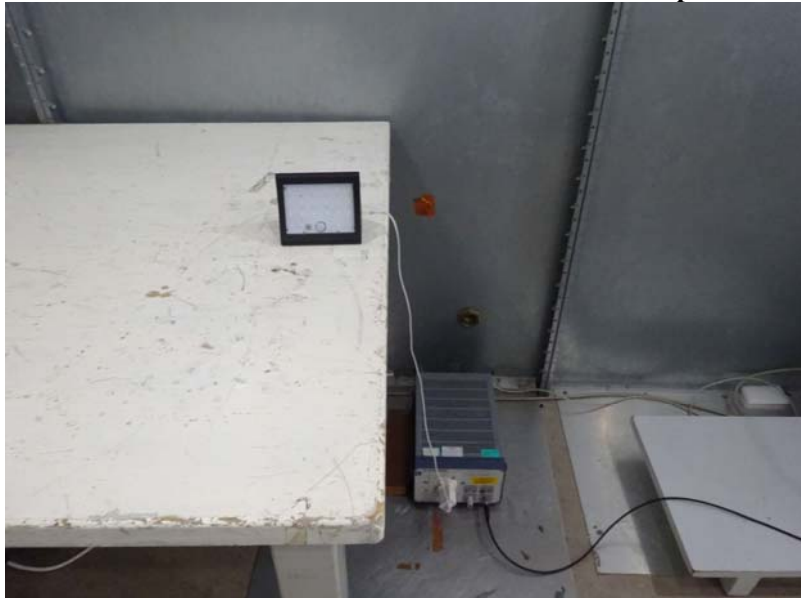
Measurement of Conducted Emission Test Set Up
