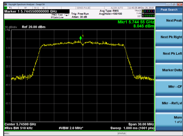
(802.11ac20) PSD plot on channel 149
