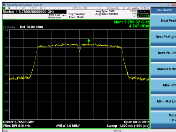
(802.11ac40) PSD plot on channel 159
