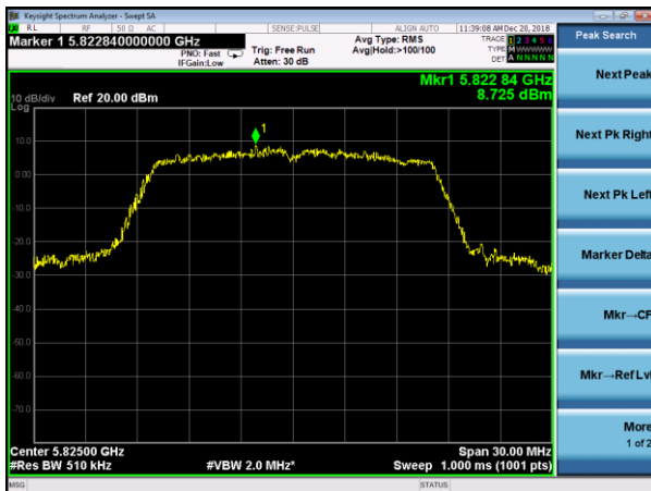
(802.11a) PSD plot on channel 165
