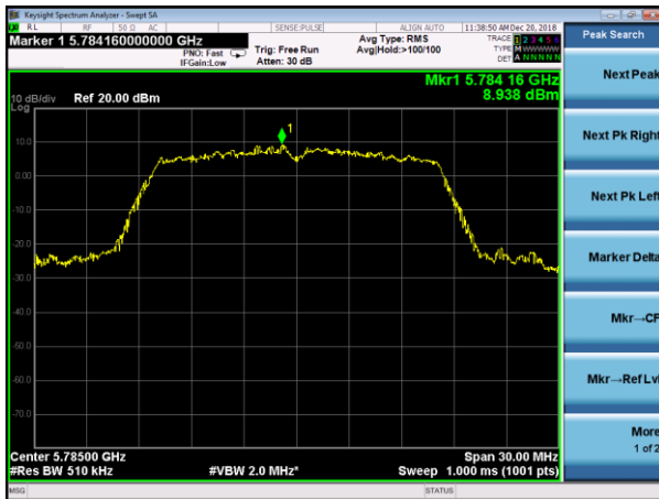
(802.11a) PSD plot on channel 157
