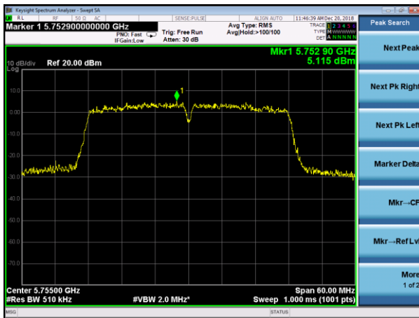
(802.11n40) PSD plot on channel 151
