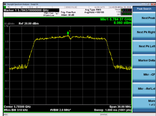
(802.11ac20) PSD plot on channel 157
