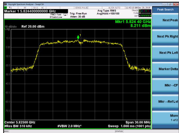
(802.11n20) PSD plot on channel 165
