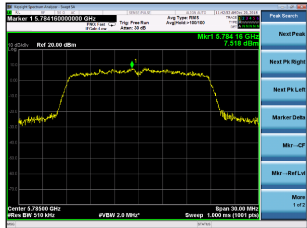
(802.11n20) PSD plot on channel 157
