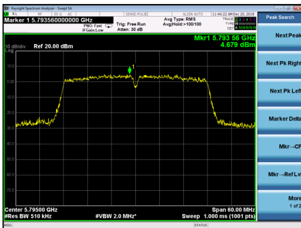
(802.11n40) PSD plot on channel 159
