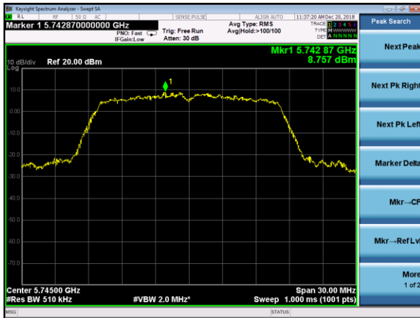
(802.11a) PSD plot on channel 149
