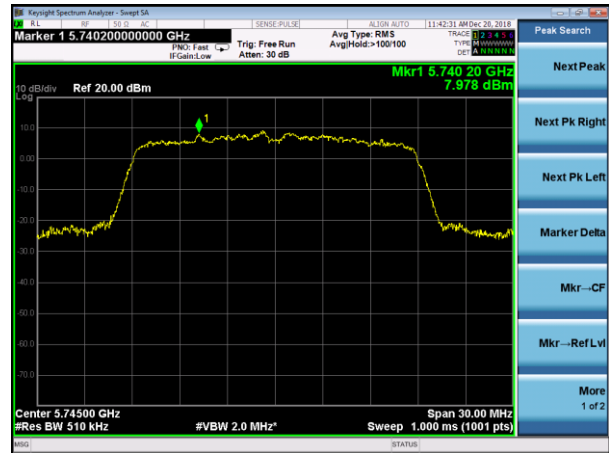
(802.11n20) PSD plot on channel 149
