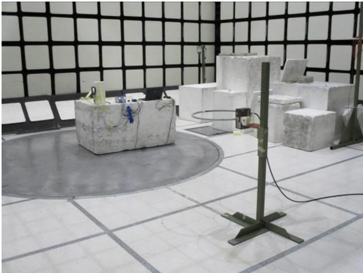
**RADIATED EMISSION BELOW 30 MHz – TX Rod Upright, RX Loop X**
