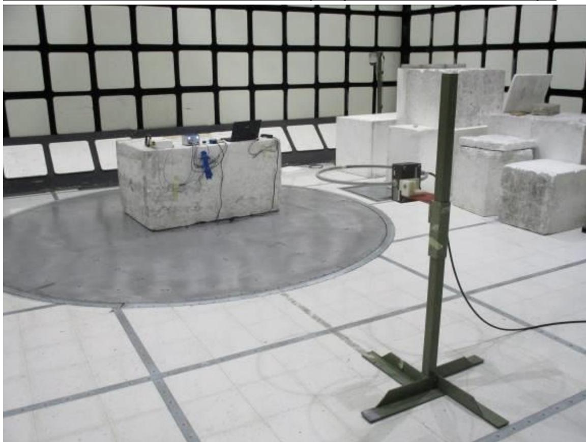
**RADIATED EMISSION BELOW 30 MHz – TX Loop Upright, RX Loop X**
