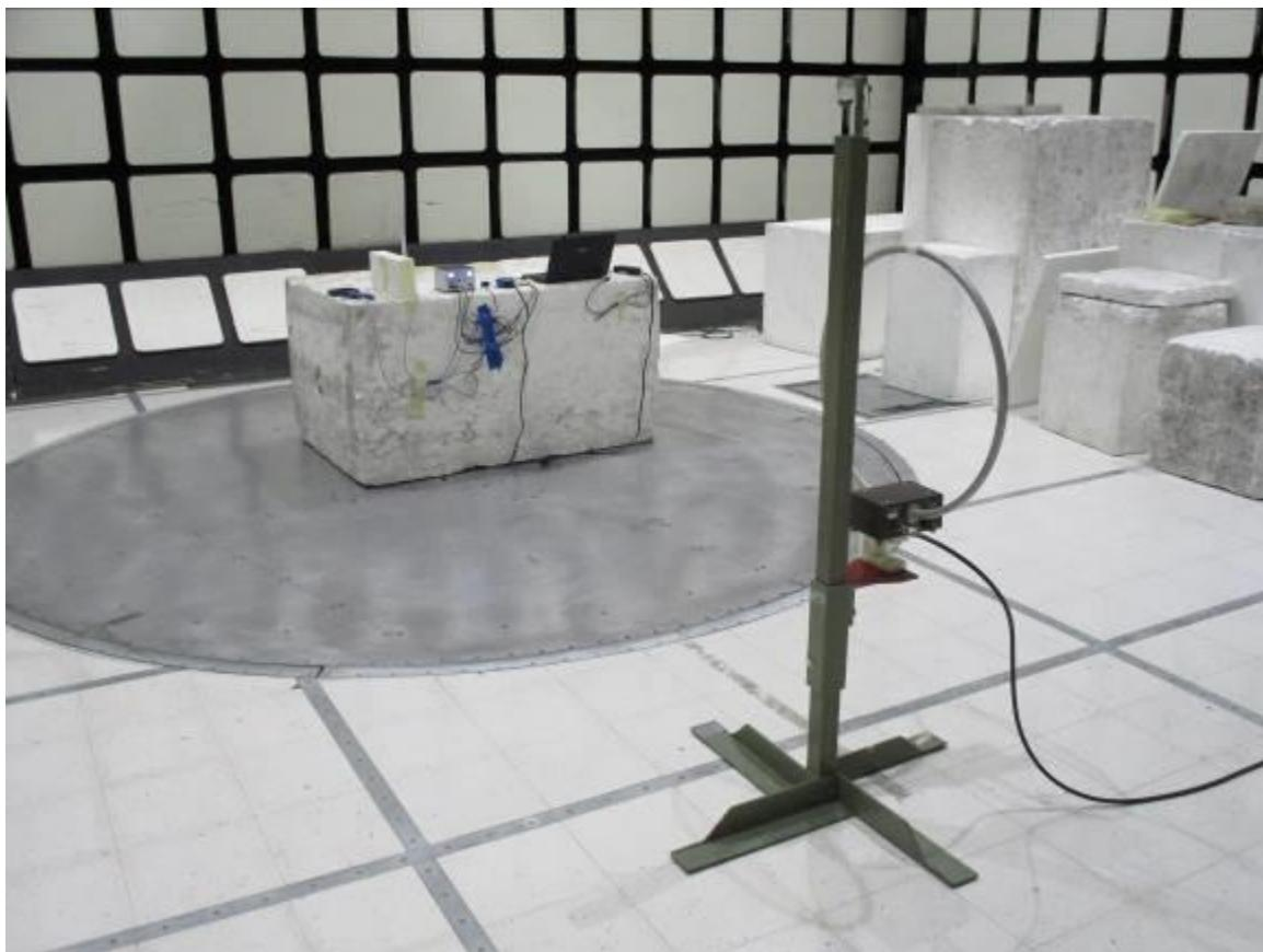
**RADIATED EMISSION BELOW 30 MHz – TX Rod Upright, RX Loop Z**
