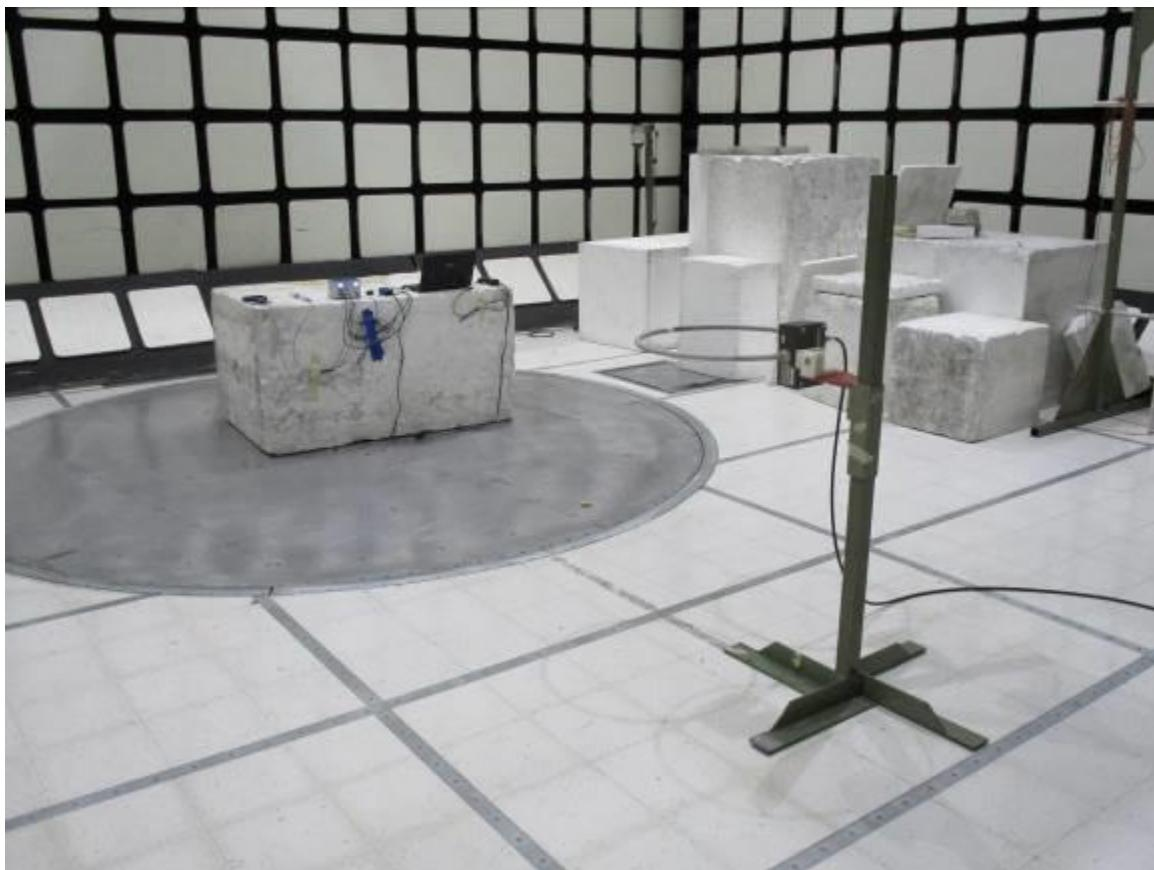
**RADIATED EMISSION BELOW 30 MHz – TX Loop Perpendicular to Ground, RX Loop X**
