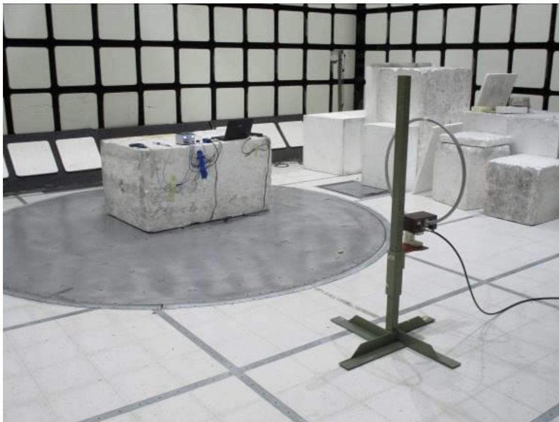
**RADIATED EMISSION BELOW 30 MHz – TX Loop and Rod Parallel to Ground, RX Loop Z**
