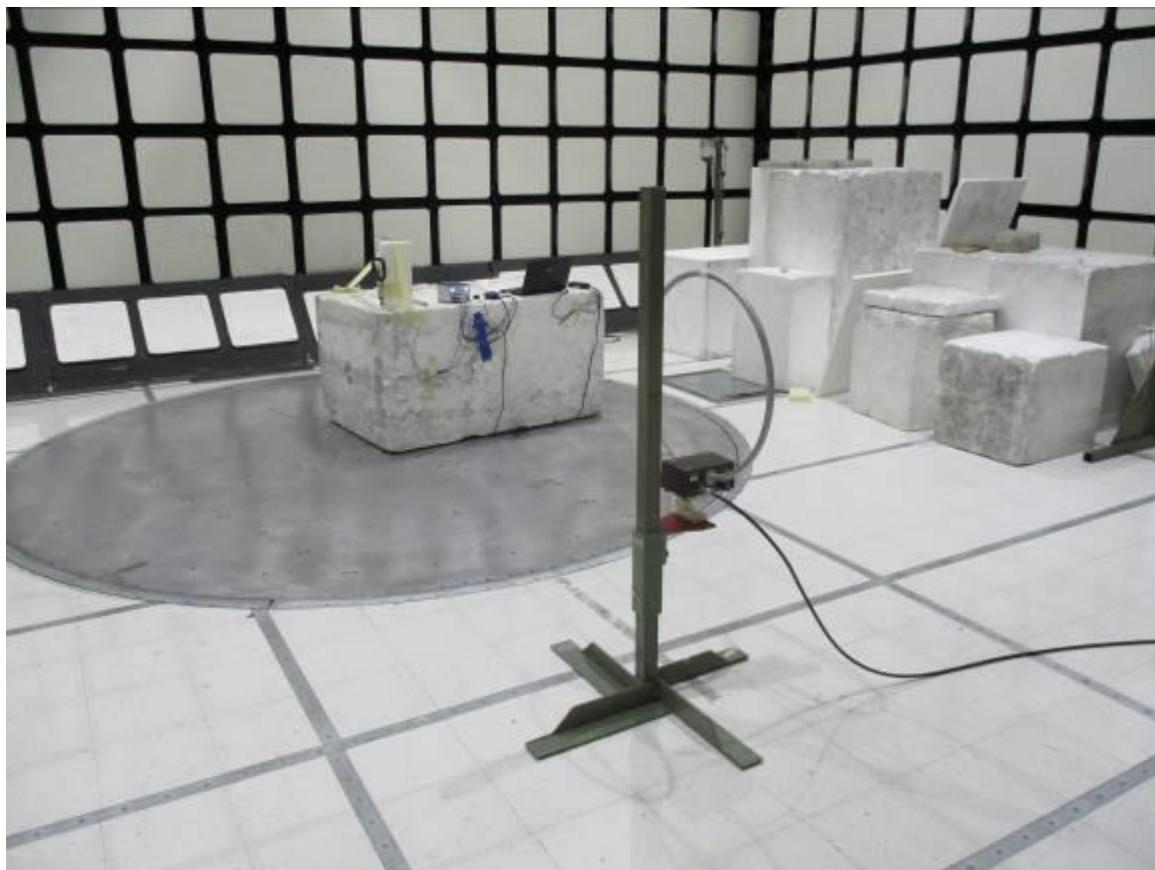
**RADIATED EMISSION BELOW 30 MHz – TX Loop Upright, RX Loop Z**
