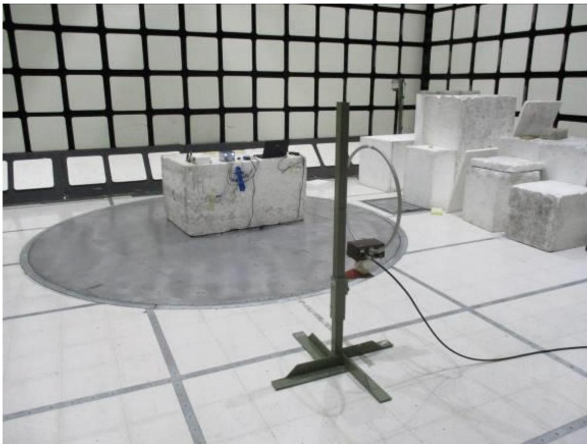
**RADIATED EMISSION BELOW 30 MHz – TX Loop Perpendicular to Ground, RX Loop Z**
