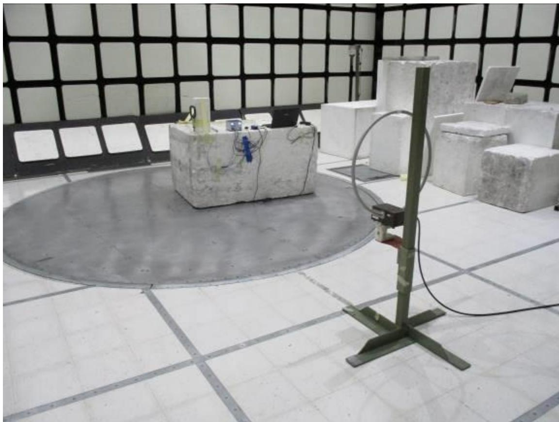
**RADIATED EMISSION BELOW 30 MHz – TX Loop Upright, RX Loop Y**
