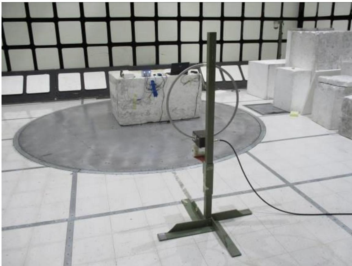
**RADIATED EMISSION BELOW 30 MHz – TX Loop Perpendicular to Ground, RX Loop Y**
