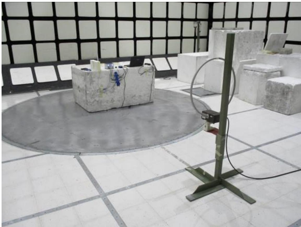
**RADIATED EMISSION BELOW 30 MHz – TX Rod Upright, RX Loop Y**
