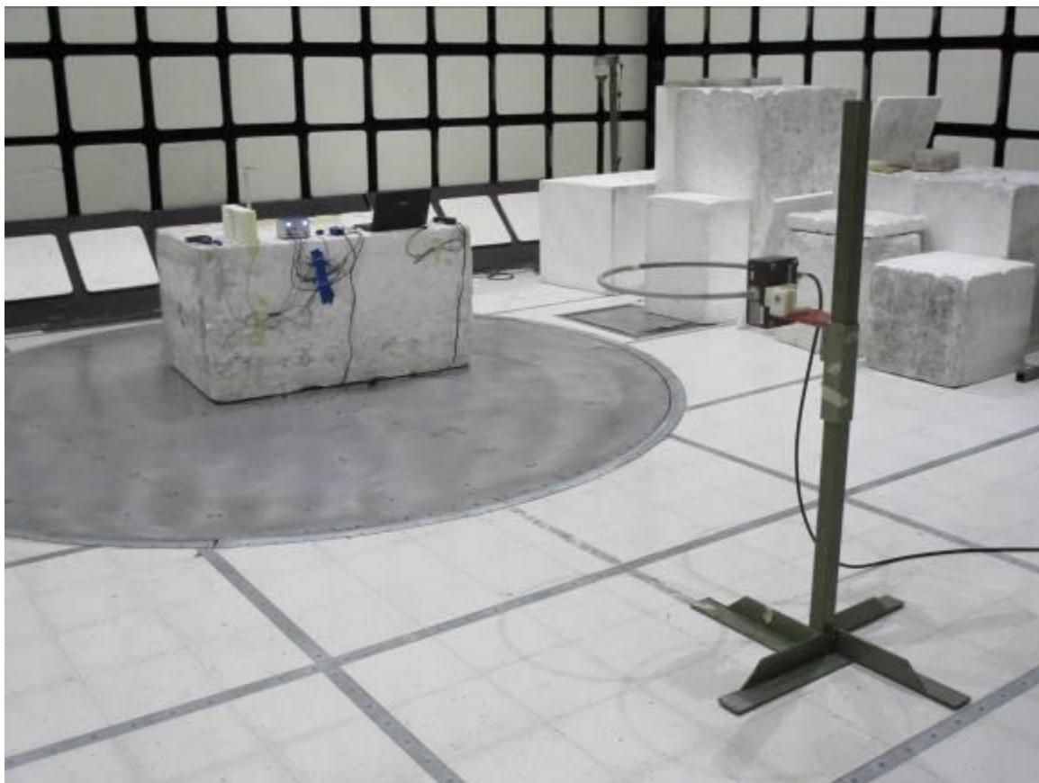
**RADIATED EMISSION BELOW 30MHz – 1GHz General Setup**
