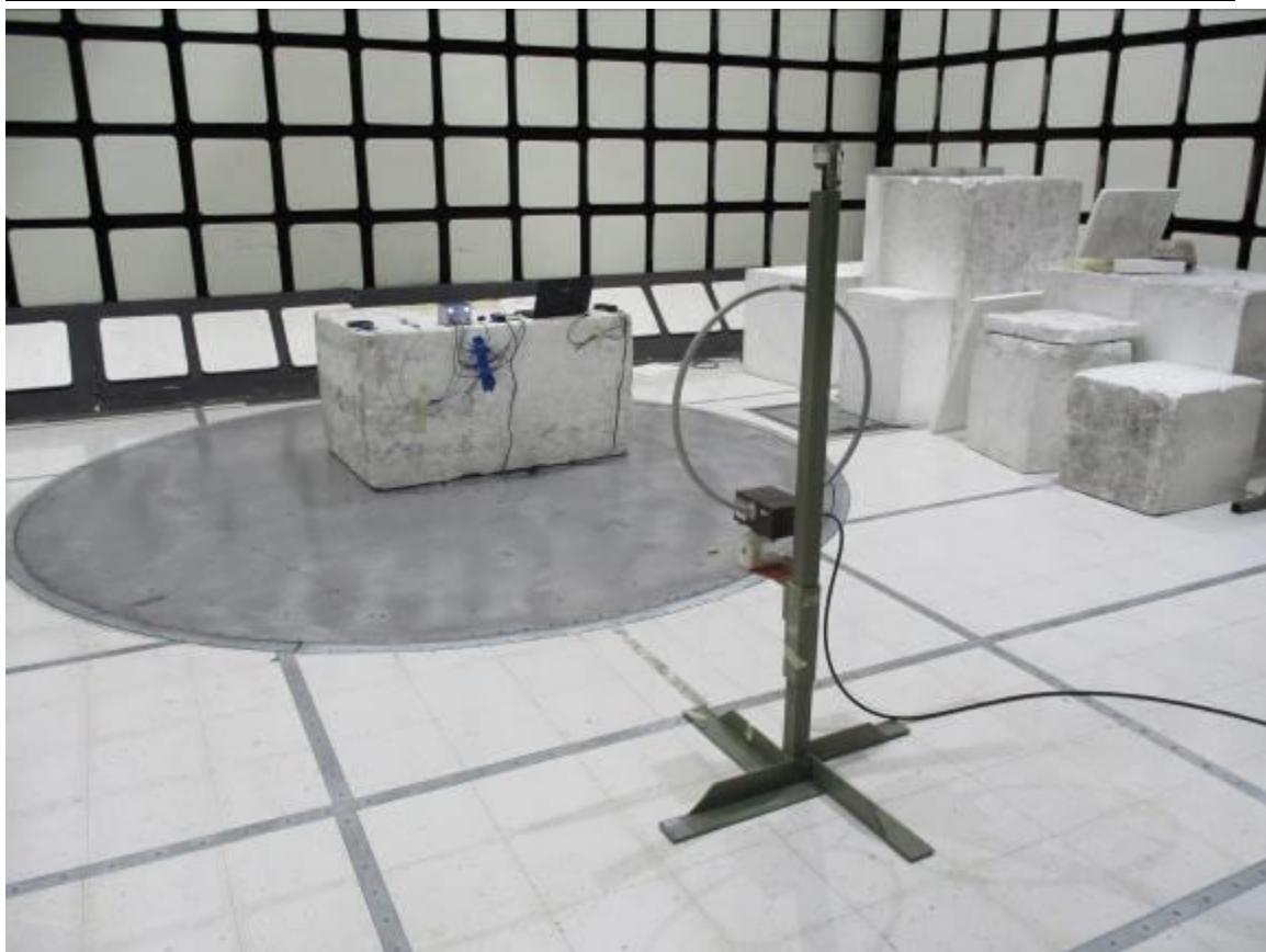
**RADIATED EMISSION BELOW 30 MHz – TX Loop and Rod Parallel to Ground, RX Loop Y**
