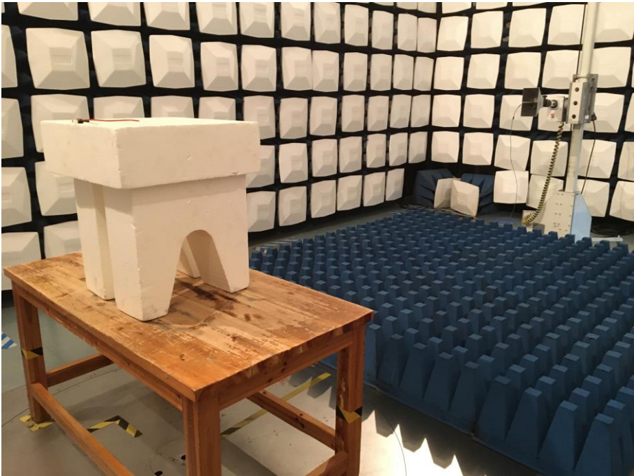
Test Setup For Radiated Emission (Above 1GHz)
