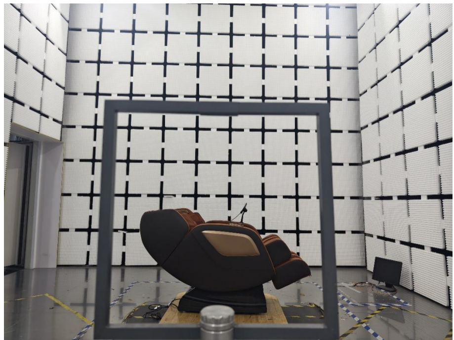
Radiation Emission Test Setup (Below 30MHz)
