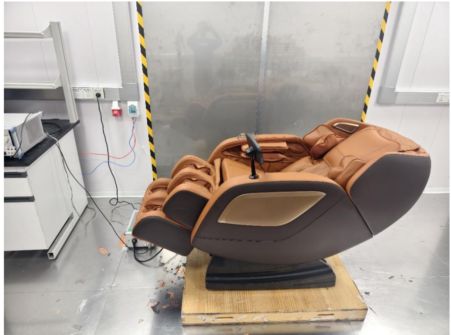
Conducted Emission Test Setup
