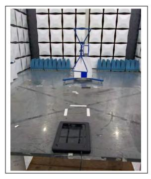
Radiated Spurious Emissions, 1 GHz to 18 GHz
