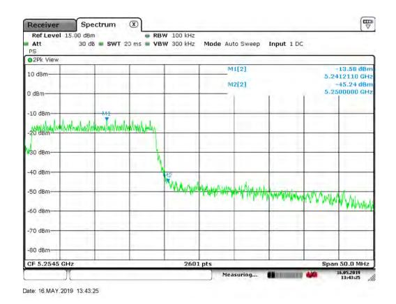
MeasurementLimit40 MHz, Lower Band Edge-37.27dBm/MHz-27dBm/MHz40 MHz, Upper Band Edge-45.24dBm/MHz-27dBm/MHz
