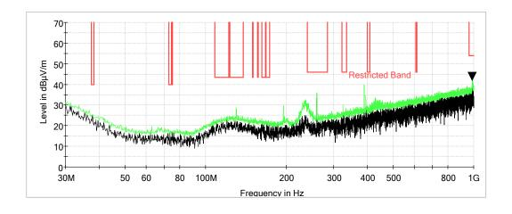
Note: There were no emissions from the EUT in any restricted band within 20dB of the limit from 9kHz to 1GHz, and no peak emissions were within 10dB of the Quasi-Peak limit.
