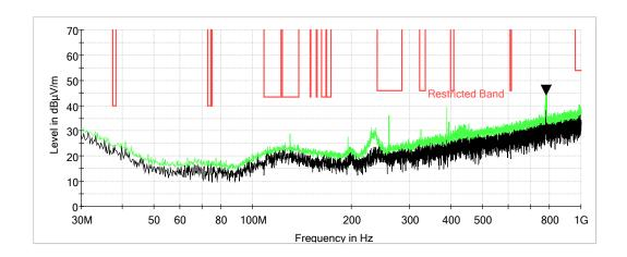
Note: There were no emissions from the EUT in any restricted band that were within 20dB of the limit from 9kHz to 1GHz, and there were no peak emissions were within 10dB of the Quasi-Peak limit.
