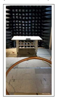
Radiated Spurious Emission, Less Than 1 GHz
