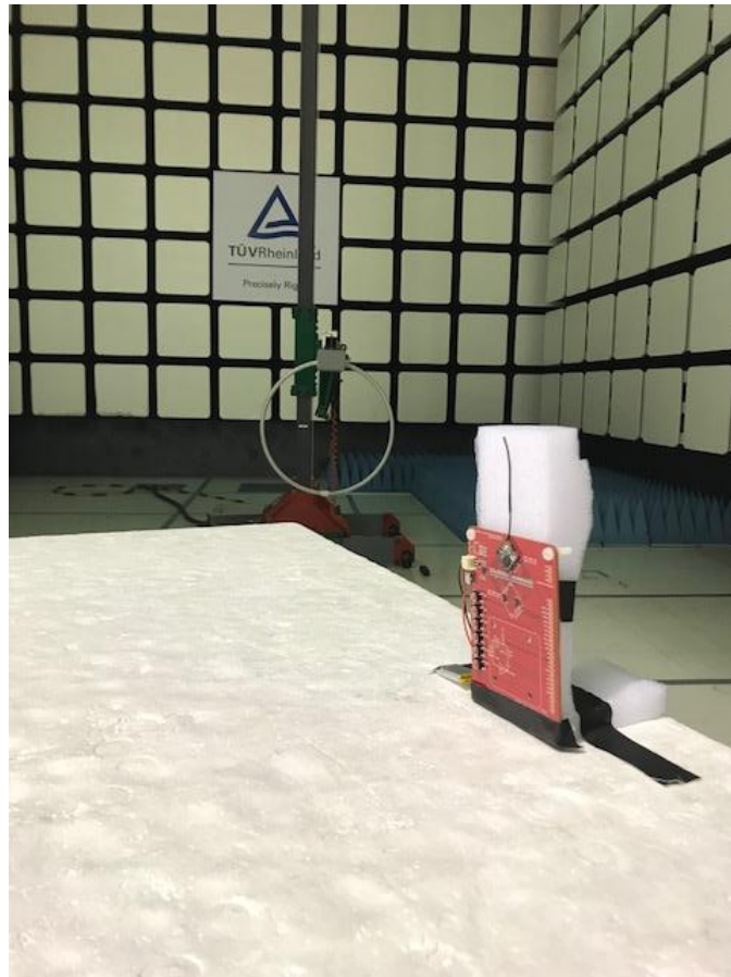
Figure 1: Test Setup for 9 kHz to 30 MHz (Front View)
