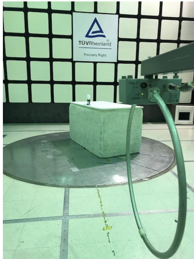
Figure 2: Test Setup for 9 kHz to 30 MHz (Rear View)
