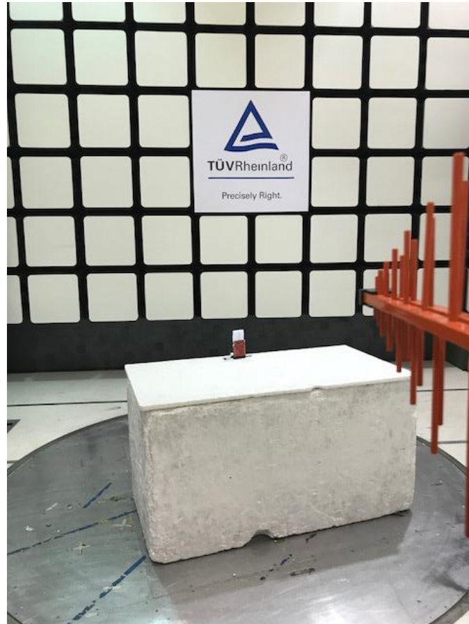
Figure 4: Test Setup for 30 MHz to 1000 MHz (Rear View)
