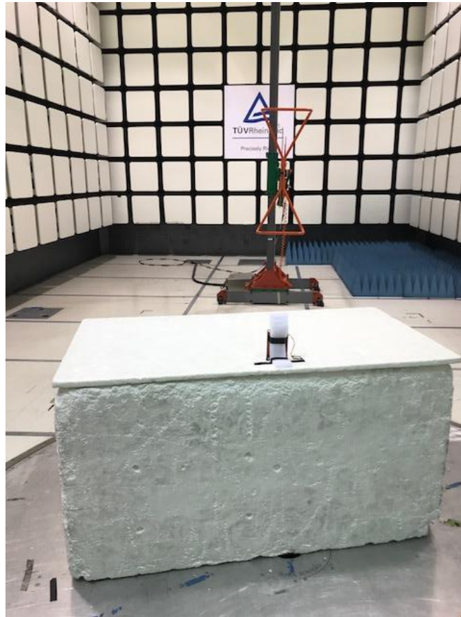
Figure 3: Test Setup for 30 MHz to 1000 MHz (Front View)
