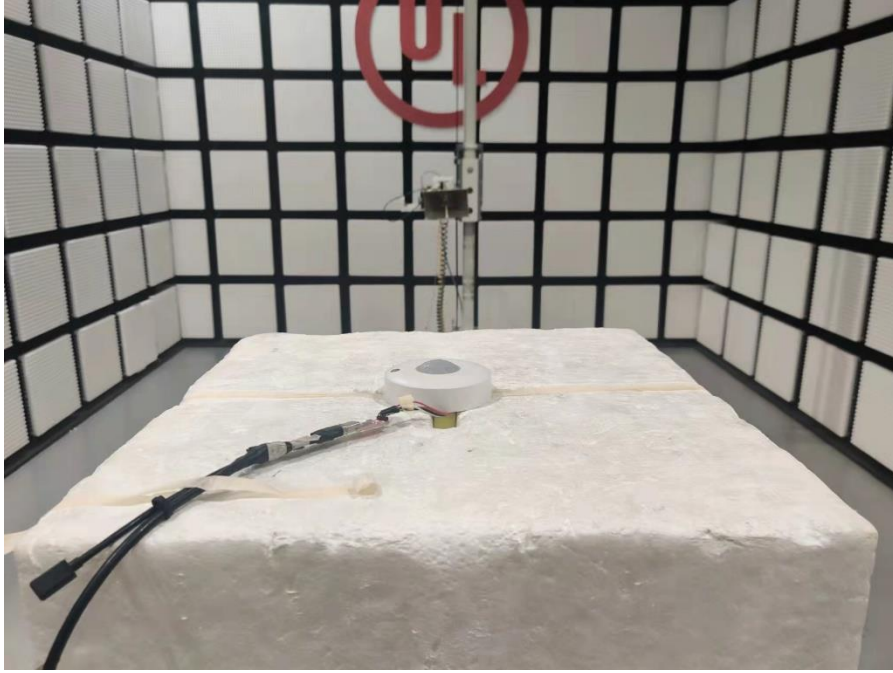
RADIATED RF MEASUREMENT SETUP (ABOVE 1 GHz) MEASUREMENT POSITION (X axis)
