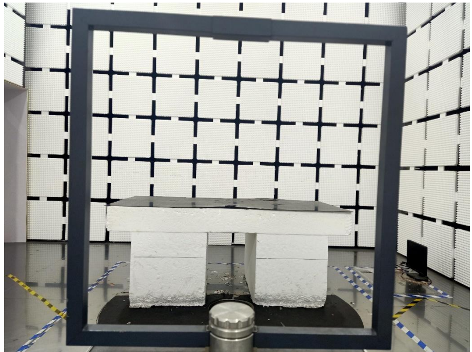
Radiation Emission Test Setup (Below 30MHz)
