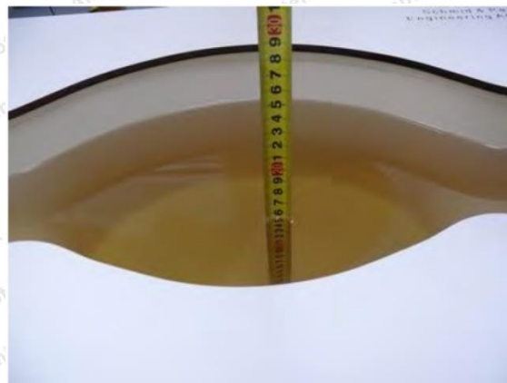
Liquid depth in the body phantom (900MHz)
