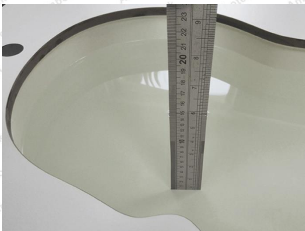
Liquid depth in the head phantom (2450MHz)
