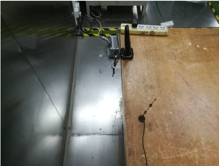
Conducted Emissions - Side View(Adapter: BLJ05W060040P-UA)
