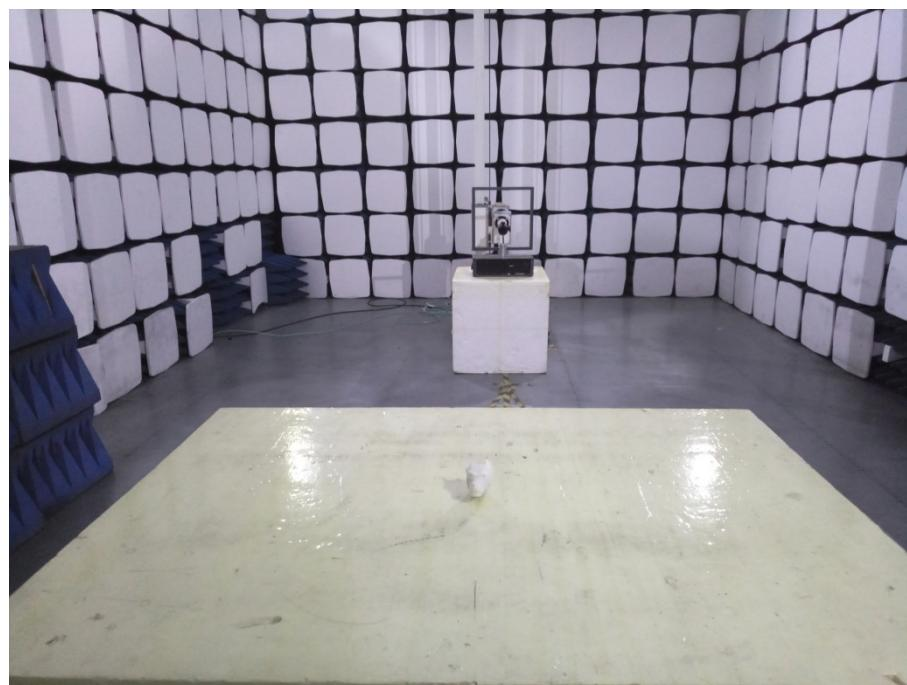
**Radiation Emission Test Setup (30MHz to 1GHz)**
