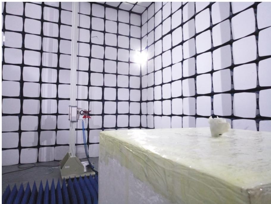
**Radiation Emission Test Setup (Above 18GHz)**
