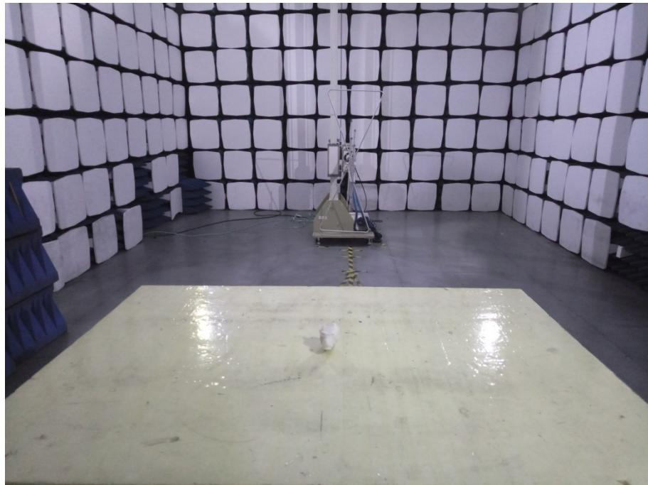
**Radiation Emission Test Setup (1GHz to 18GHz)**
