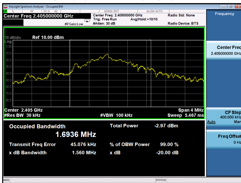
TEST PLOT OF BANDWIDTH FOR LOW CHANNEL
