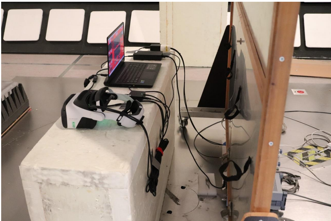
Photograph 1. Test setup for Conducted emissions 150 kHz – 30 MHz
