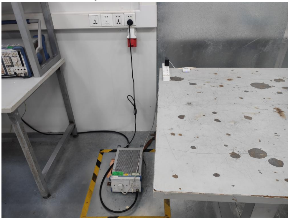
FCC ID: 2ARNO-VAR11N-300 Photo of Conducted Emission Measurement
