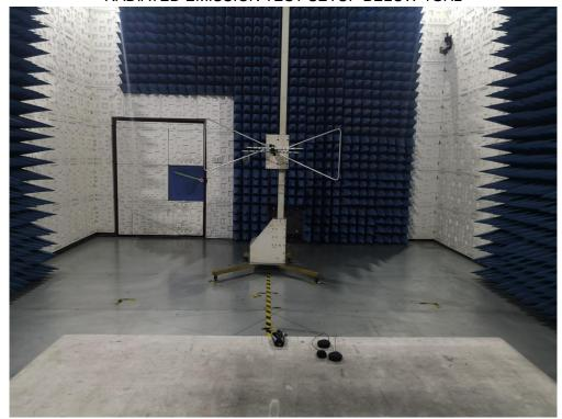
RADIATED EMISSION TEST SETUP ABOVE 1GHz
