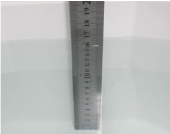
Liquid Height for Head SAR
