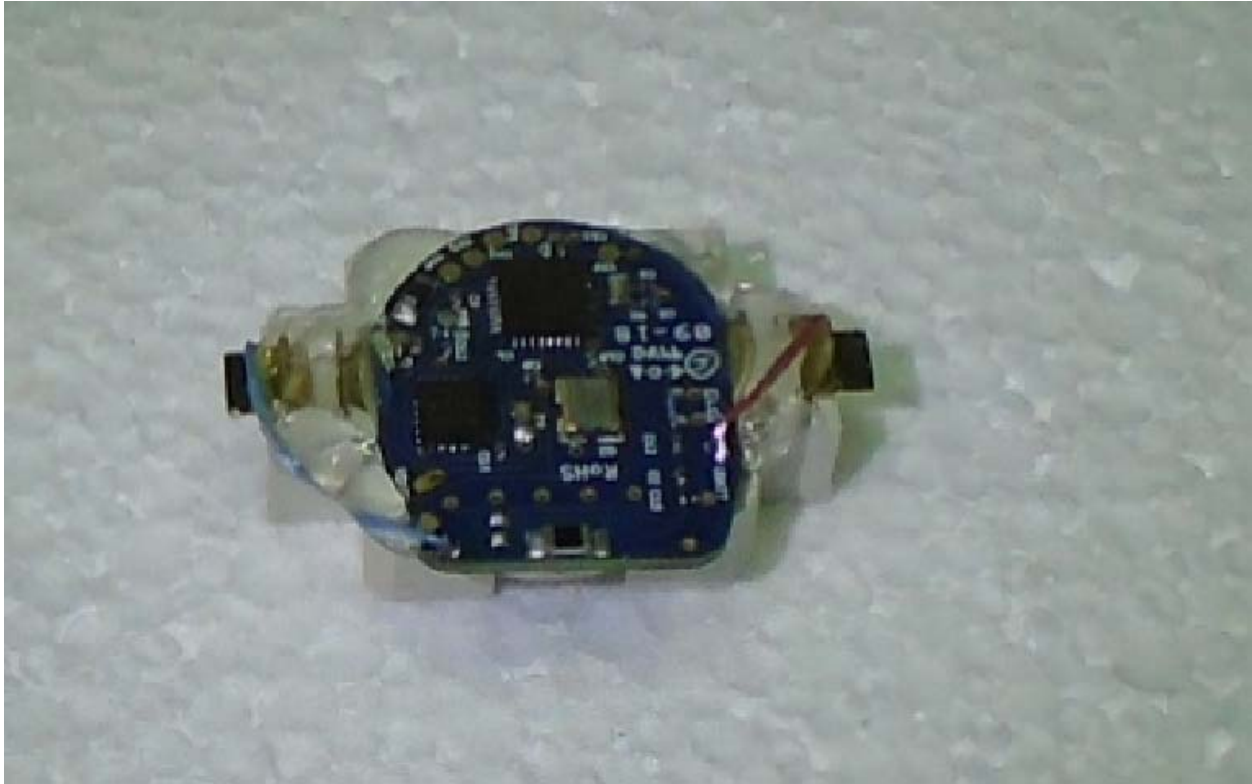
Figure 9: Radiated Emissions – Orientation C (Investigation for highest emissions)
