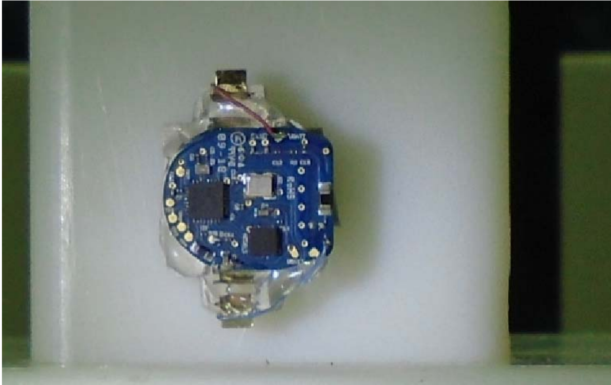
Figure 8: Radiated Emissions – Orientation B (Worst-Case Emissions)
