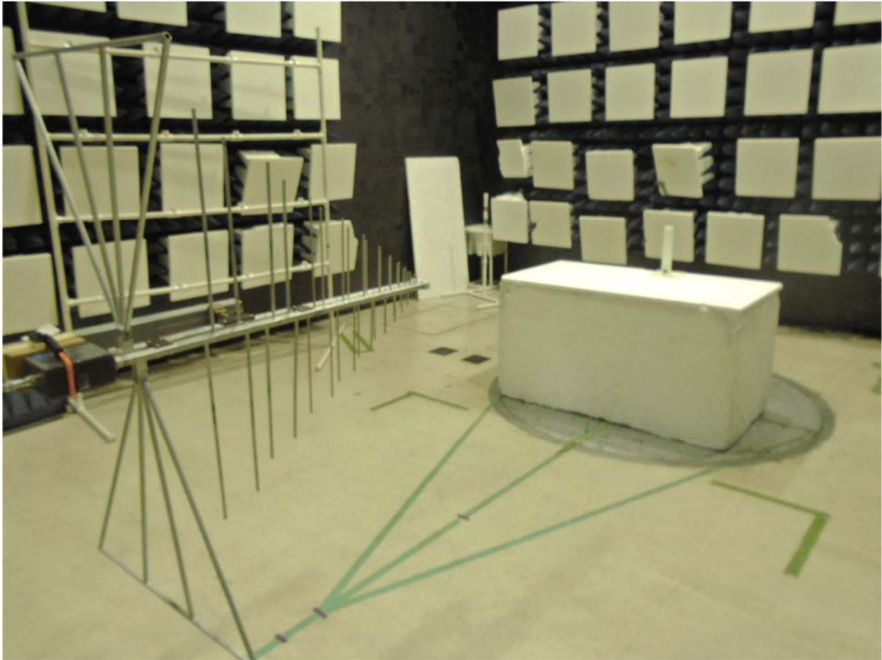
Figure 3 - Radiated Emissions Test Setup – 30 MHz to 1 GHz (5meter Semi-Anechoic)
