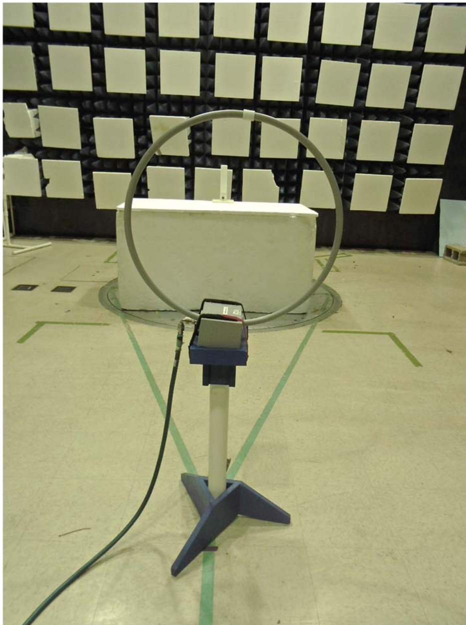
Figure 1: Typical Radiated Emissions – 10 kHz to 30 MHz Parallel Position
