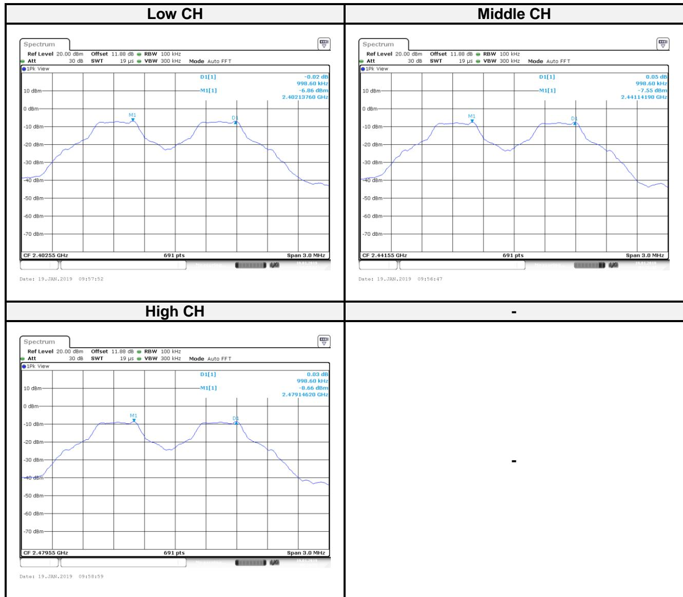
**EDR-2Mbps mode ( $\pi/4$ -DQPSK):**
