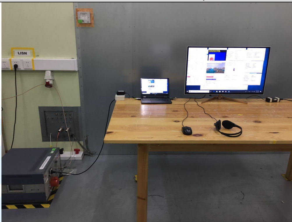
Conducted Emission Test Setup
