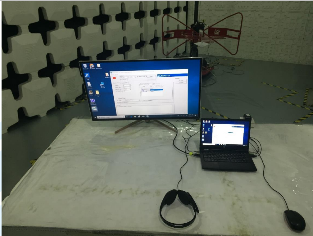
Radiated emission Test Setup (30 MHz~1 GHz)
