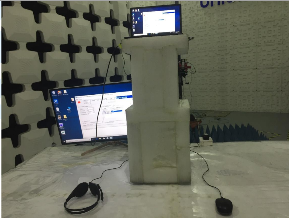
Radiated emission Test Setup (Above 1 GHz)
