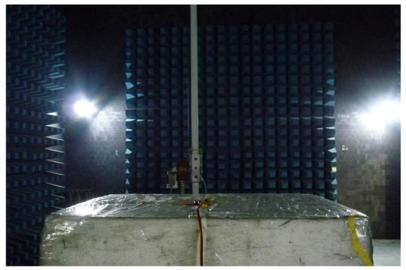
Radiated Emission Set up Photos (Front View)
