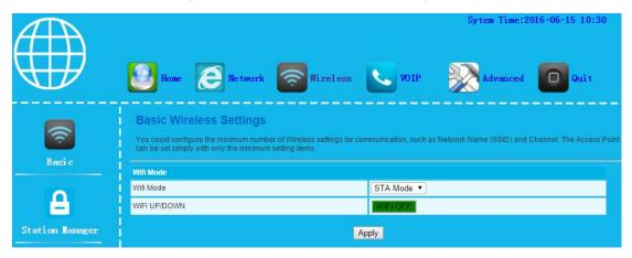
Enter Wireless Station Manager, users can view wireless connection state of equipment under STA mode, and its name and address and so on; users can also make Wi-Fi scanning and allocate required Wi-Fi.
