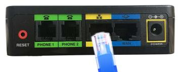
E: Connect one end of another Ethernet cable to the ETHERNET port of phone adapter. Connect
