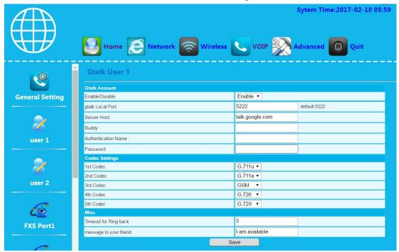
Codec Settings uses for setting the way of speech coding and can select G.711a/u, GSM, G.726, G.729, which is same as SIP.
