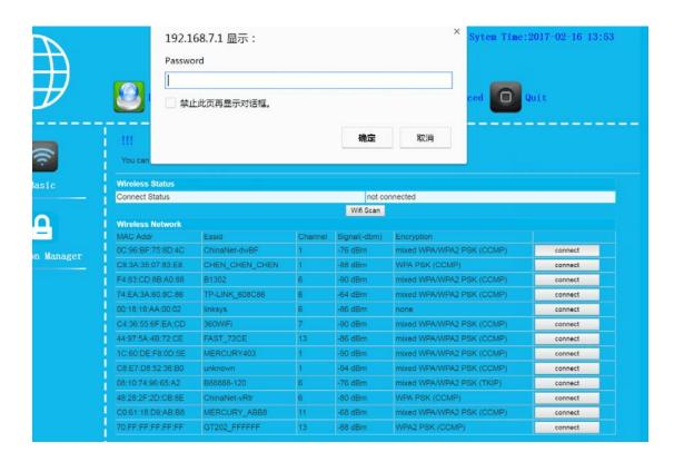
If the wrong password cause the connection fail, the web interface will display the following hint.
