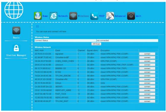
Click "connect" in the back of relevant Wi-Fi name, then input relevant password according to hint, and the equipment will begin to connect Wi-Fi.
