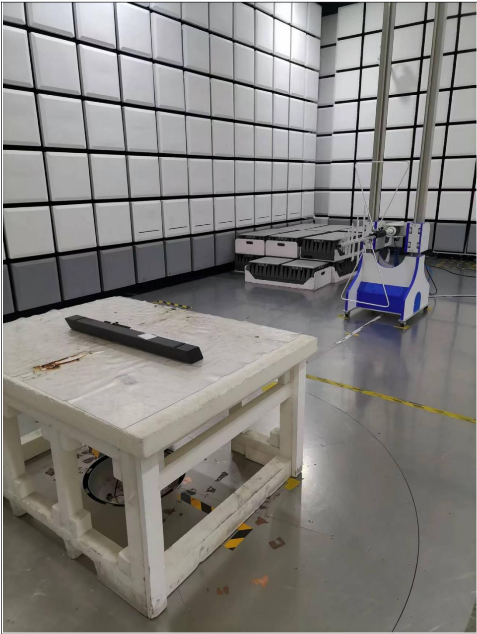
RADIATED EMISSION TEST (Below 1GHz)
