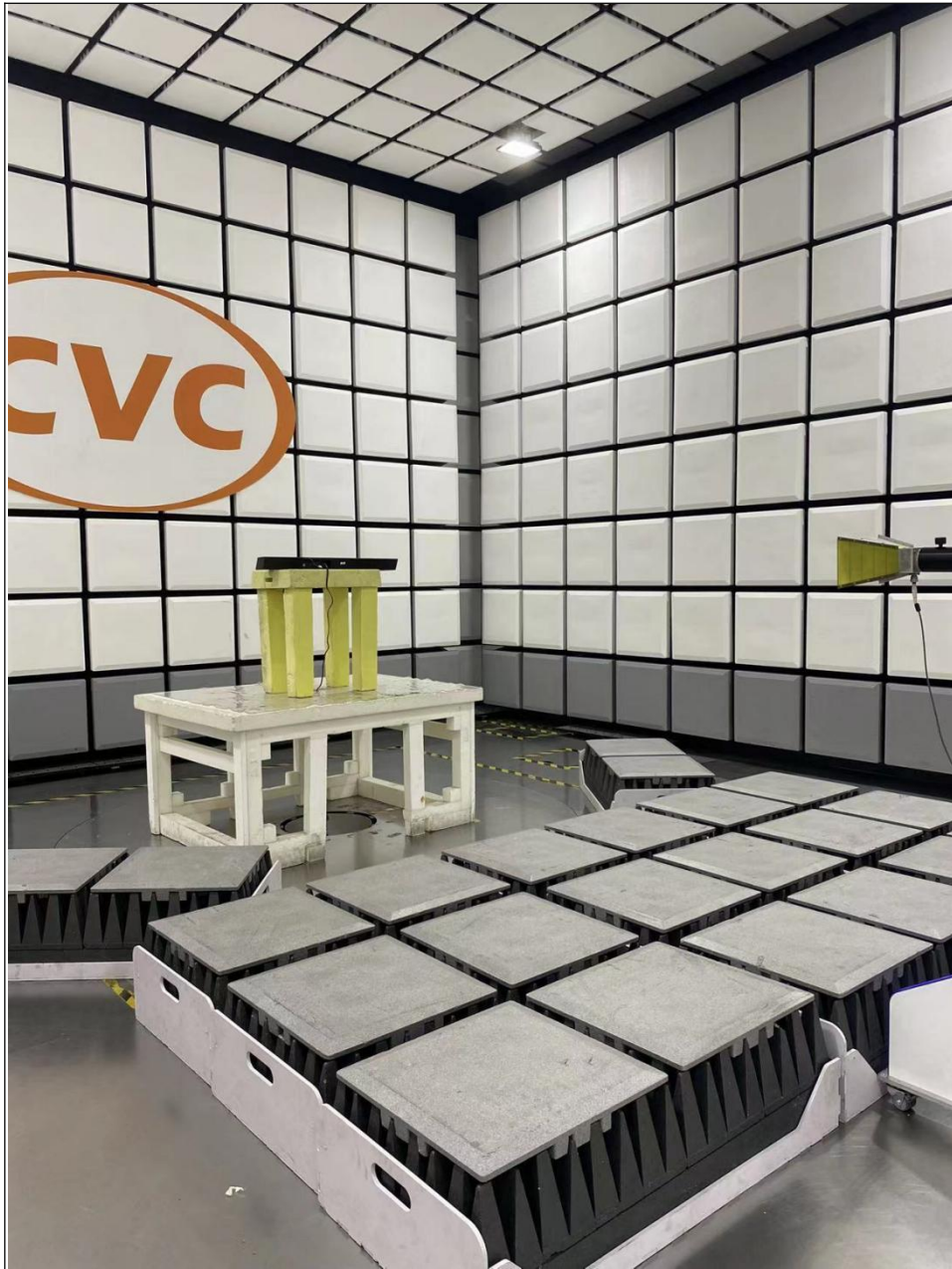
RADIATED EMISSION TEST (Above 1GHz)
